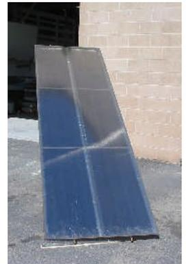
These new glazed pool collectors are designed to heat pools when ambient temperatures are below the desired pool temperature by up to 60 F. It limits temperature, probably topping off at 270 F instead of over 400 F like conventional 40 s/f collectors. The Black Crystal absorber increases low-end performance. About 50 to 80% of pool area is needed in collector area depending on needs.
